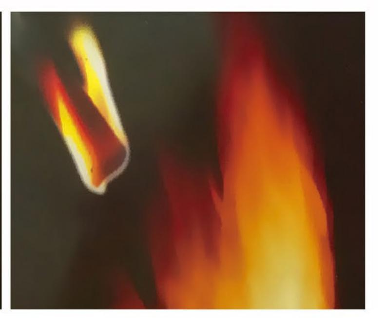
Class B flame has generated Normal PE core ACP(combustible)
